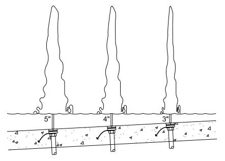
The XFJ20 Series jets can also be installed in the pool floor, in a beach entry, shallow swim out or kiddy area. The jet is adjusted vertically and shoots up through the pool water creating an aerated stream. The jet requires more gallonage at higher head pressures when used under water then as a deck jet to achieve the same height. The deeper in the water, the higher the requirements. The shallower depths may cause the jet to bounce up and down due to the wave action of the surface.
