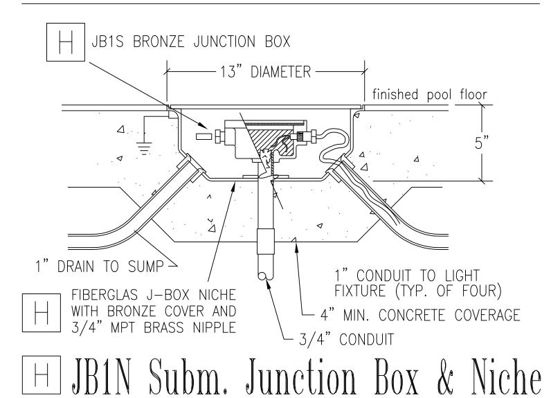
N.T.S. Typical Installation Detail
